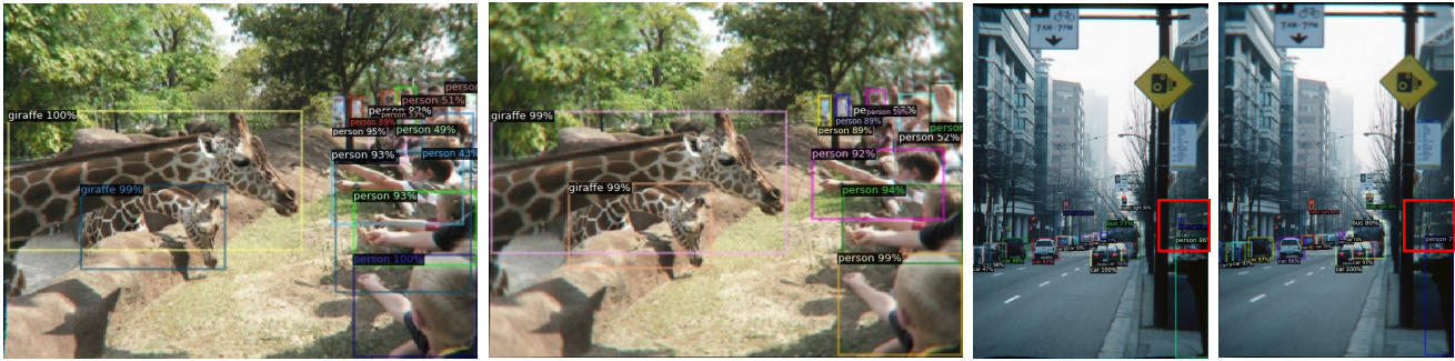
Figure 5. Qualitative object detection results. Left: TaskLens (triplet). Right: ImagingLens (triplet #1). We use the official pretrained “faster_rcnn_R_50_FPN_3x” model without fine-tuning for each lens. Left example: more people are detected in the TaskLens simulated image. Right example: the traffic light is successfully detected only in the TaskLens simulated image (marked by the red box). Moreover, detection boxes in the TaskLens render images usually have higher confidence.
