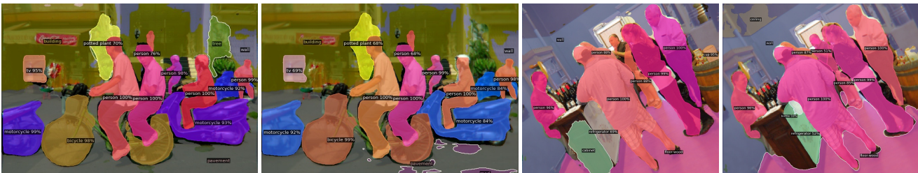
Figure 6. Panoptic segmentation results. Left: TaskLens (triplet). Right: ImagingLens (triplet #1). We use the official pretrained “panoptic_fpn_R_101_3x” model without fine-tuning for each lens. Segmentation results on TaskLens rendered images contain fewer artifacts. The corresponding detection results have higher confidence.
